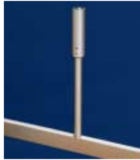
6190 Hanger rod Gives height and level adjustment by moving hanger rod within 6192 sleeve. When in position the hanger is firmly fixed to the rail by 6194 insert and to the ceiling by 6193 stud.
