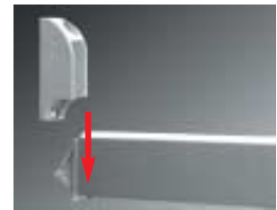
Wall support after downward separation
