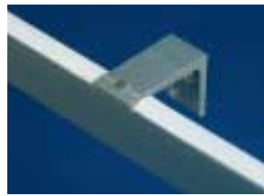
6503 Wall bracket Used where rail is to be fixed parallel to the wall. Bracket is screwed to the wall, rail slots in and screw secures from above. Anodised aluminium, available in 4 widths and 2 different projections depending on usage.
